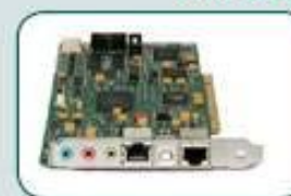
IP Communication Card 175.26mm x 100mm
