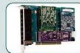
VoIP Gateway Card 165mm x 100mm
